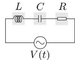
Fig.4. An LC series circuit with a resistor R.
