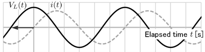
Fig.1. The curve for the voltage drop at a coil which shifts toward the past time.
