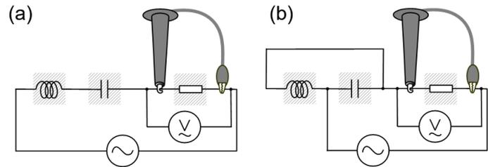
Fig.8. An LC series circuit (a) and parallel circuit (b) by use of the LCR block.
