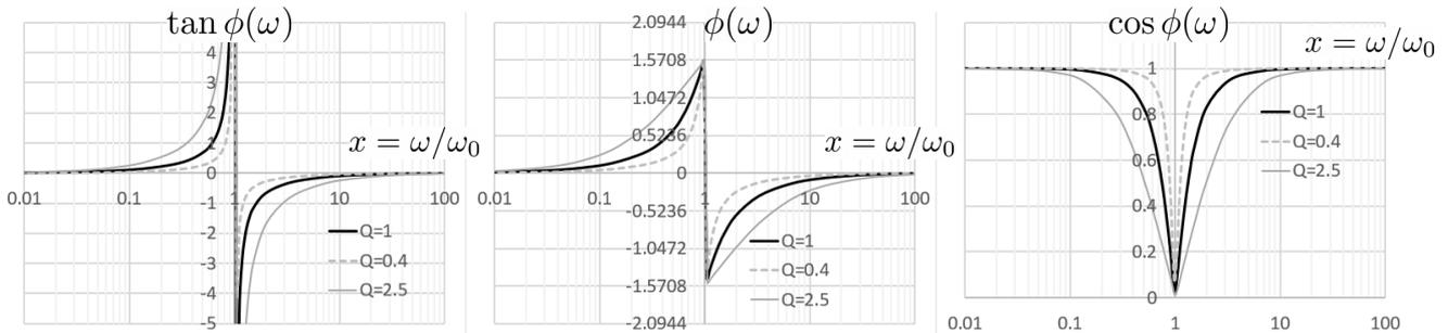
Fig.7. The frequency dependence of  $\tan \phi$ ,  $\phi$ ,  $\cos \phi$  for LC parallel circuit. The horizontal axis in those graphs is  $x = \omega\sqrt{LC}$  in a log scale.
