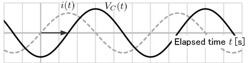
Fig.2. The curve for the voltage drop at a capacitor which shifts toward the future.
