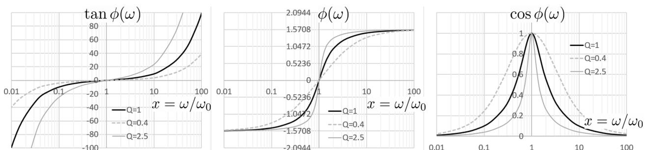
Fig.5. The frequency dependence of  $\tan \phi$ ,  $\phi$ ,  $\cos \phi$  of LC series circuit. The horizontal axis of those graphs are  $x = \omega\sqrt{LC}$  in a log scale.
