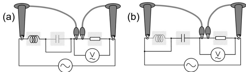
Fig.3. Usage of LCR block for LR circuit (a) or CR circuit (b).
