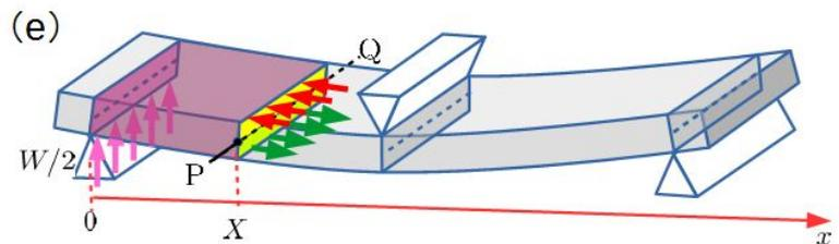
Fig.2-3 Torque balance of a part (0 to  $x+dx$ )
