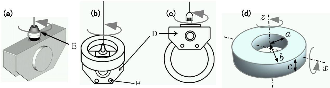
**Fig. 3-2 (a) A fitting for the bottom of the wire. (b) A weight placed horizontally on the fitting and (c) the same weight hunged vertically. (d) The dimensions of the ring-shaped weight.**
