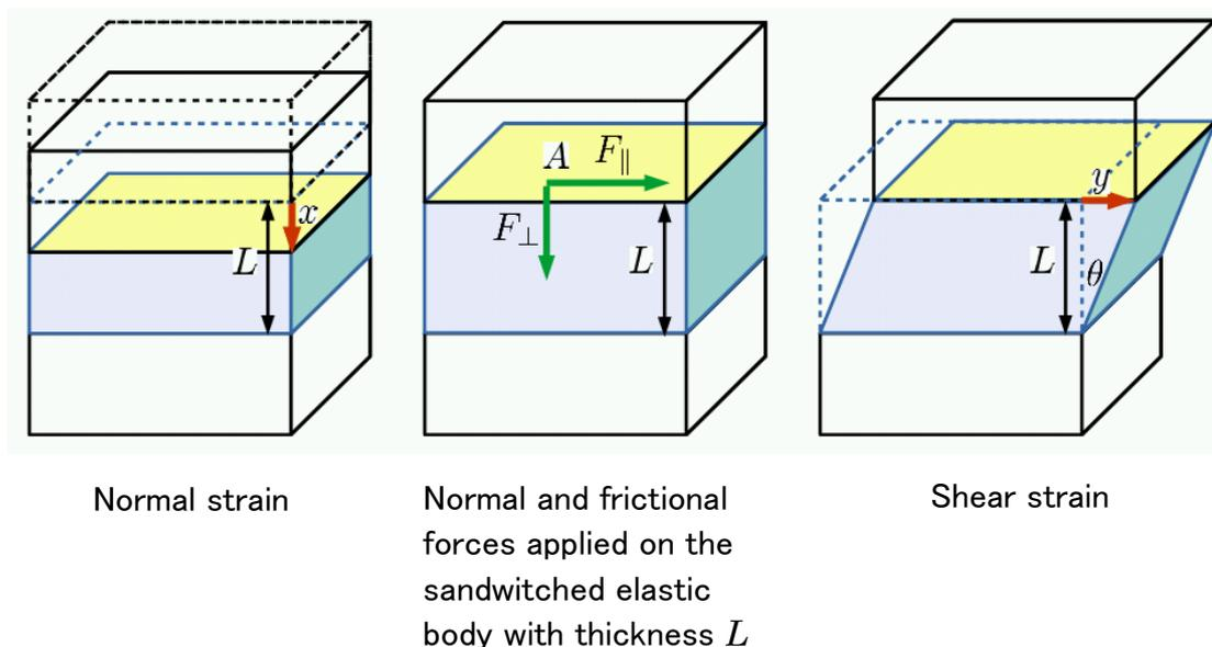
Fig. A-1 Normal and shear displacements and strains by forces
