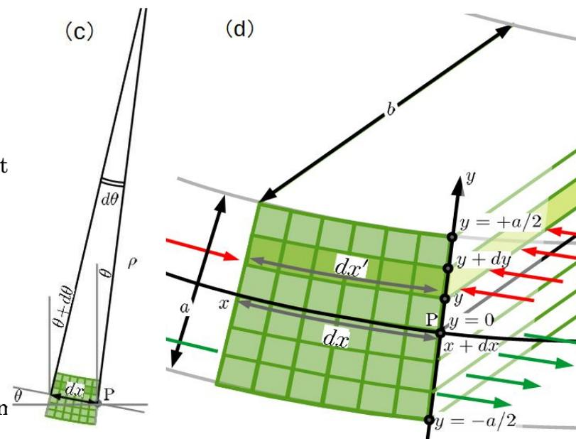
Fig.2-2 Enlarged views of the bar ( $x$  to  $x+dx$ ).
