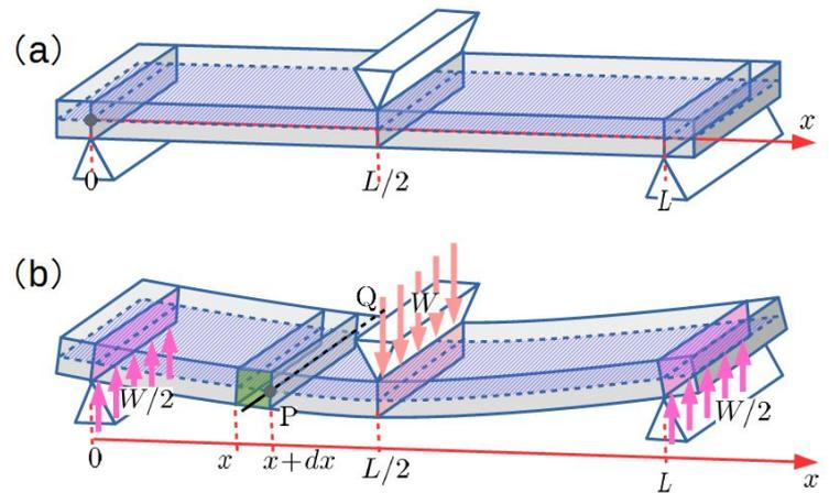
Fig.2-1 The deformation of a flat metal bar.
