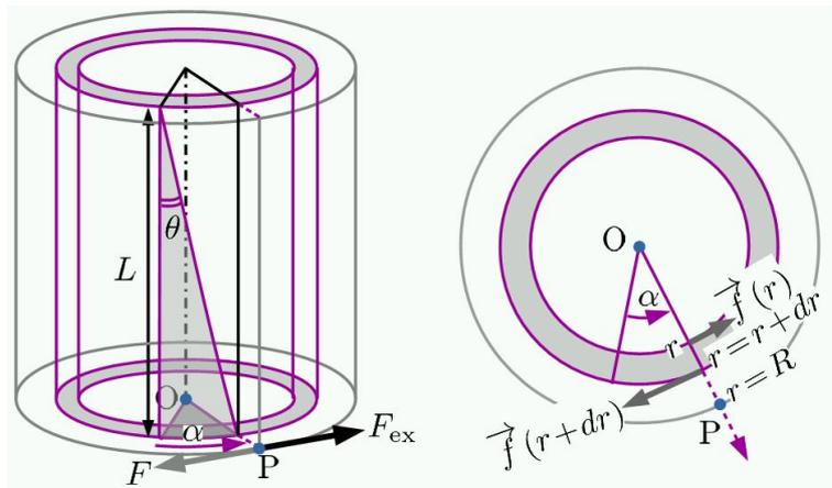
Fig. 3-1 Torsional deformation of a wire
