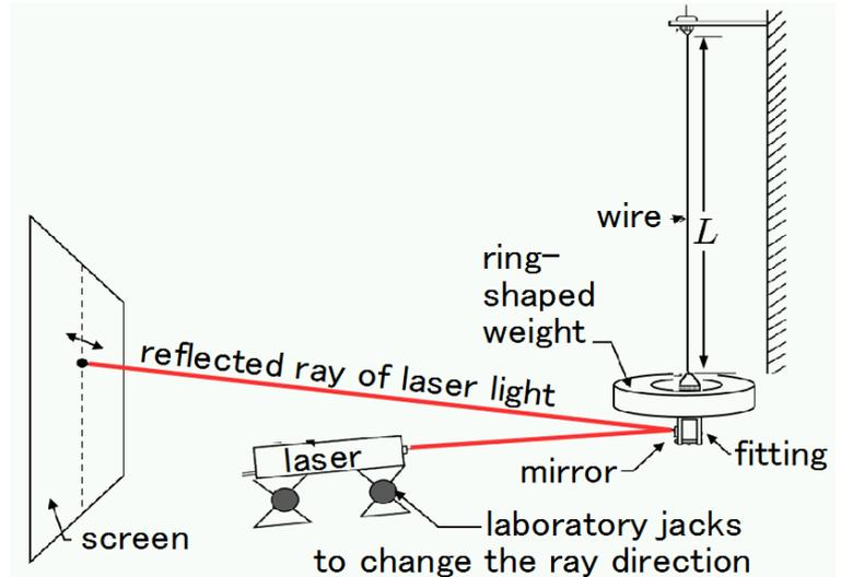
Fig. 3-3. Overall apparatus of the torsional pendulum.
